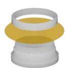
Cat. No: **1083** and **1085** are closed on one end and also integrate an external overflow reservoir and ThermoPlastic® venting option. The two sample cups are identical with the exception of their heights. The 1083 is approximately 3 mm less in height for accommodation by sulfur analyzers designed with a sample cup holder lid that requires a smaller sample cup height.
