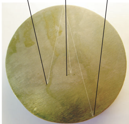
Fig. 7. \varnothing 115 mm bar. Non-metallic inclusions.
